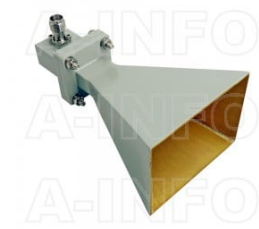
LB-90-15-C-TF Standard Gain Horn Antenna 8.2-12.4GHz 15dB Gain TNC Female
